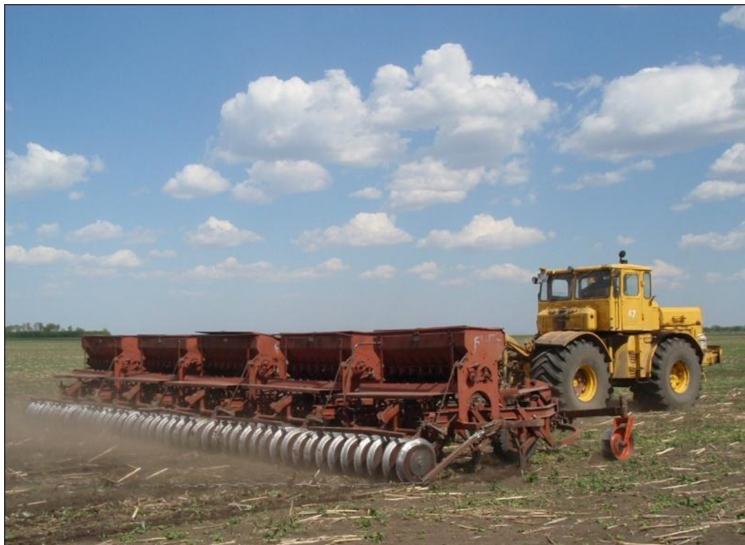
The farm has five x 30 foot Russian hoe-press drills pulled by Kirovets tractors
